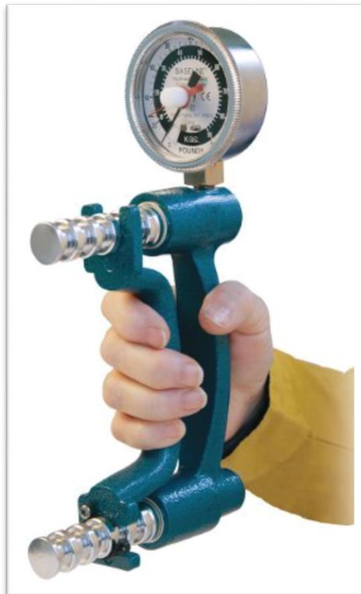
Figure 2 Hand Grip Dynamometer
