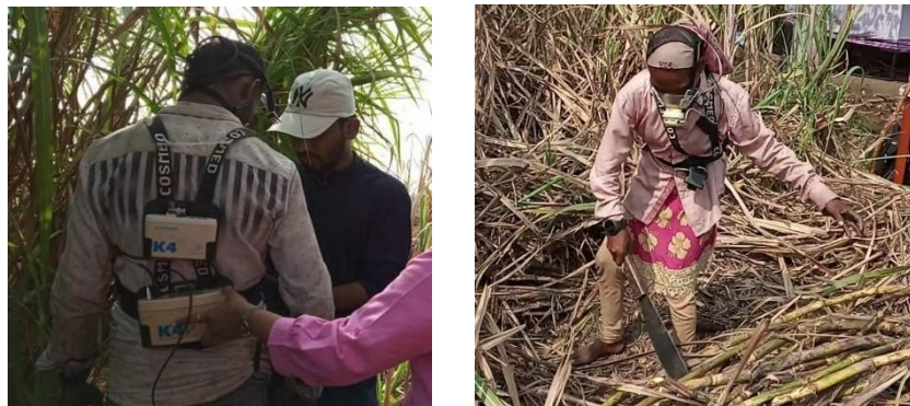
Figure 5 Measurement of Energy Expenditure using K4b2.
